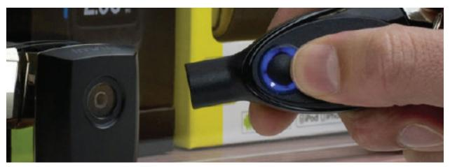
The E Ink display on InVue's OneKEY solution requires no electrical connection or battery on the retail case to show if the case is locked or unlocked.
